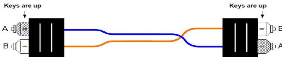
NOTE - SC connectors are shown, but this assembly may be built using any duplex single-fiber connectors or connectors with two fixed fibers that meet the requirements of a published FOCIS.
